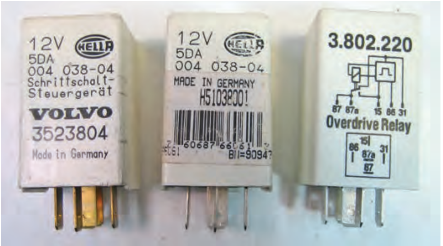
Three new relays, all of them Volvo part number 3523804. The one on the left is a Genuine Volvo relay, the middle one is an OEM Hella relay, and the right one an aftermarket relay made by K.A.E. in Germany. Note that Hella attached a sticker to cover up the scratched off "Volvo 3523804."
