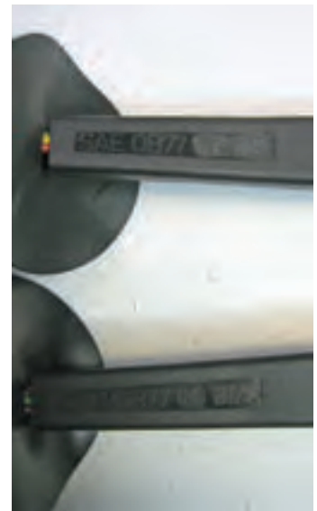
Two identical 240 cruise control switches, both NOS. One was sold by Volvo as a Genuine part. The other was sourced from a parts distributor without a brand name. Both switches were made by LK, the one sold generically has LK's logo and part number ground off, as opposed to Volvo's part number. LK may have produced these for a third party "white label" vendor, as opposed to marketing them under their own name.
