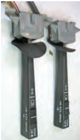
Two identical 240 cruise control switches, both NOS. One was sold by Volvo as a Genuine part. The other was sourced from a parts distributor without a brand name. Both switches were made by LK, the one sold generically has LK's logo and part number ground off, as opposed to Volvo's part number. LK may have produced these for a third party "white label" vendor, as opposed to marketing them under their own name.
